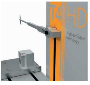
Problem: Contour- and roughness measuring devices with solid Z-columns can prevent an unobstructed view of drillings and test subjects when teaching-in the measurement programme. Longer test subjects, such as shafts or ball screw spindles, must often be cut to length for measuring to prevent collision with the measuring device.
